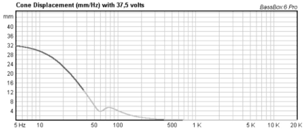
At 20 Hz the cone displacement is at maximum allowable resulting in risk of damage to the driver. If the amplifier has a subsonic filter this should be set for 30 Hz High Pass protecting the driver from overload. See green curve below.
