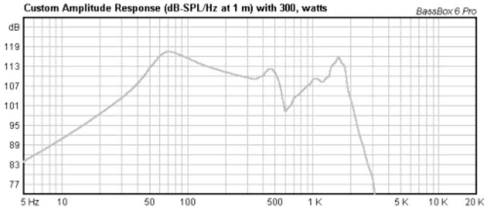
From the simulation can be seen that very high SPL above 116 dB is possible from 60 to 100 Hz. However the cone displacement is also very high below tuning, see graph below for peak displacement.
