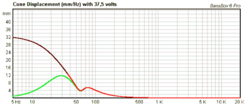
Comparing the above peak displacement curve with the red it can clearly be seen that the high pass filter (green curve) protect the driver from overload because the cone displacement is well below max in the full frequency range.
