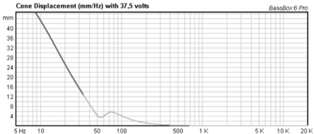
At 20 Hz the peak cone displacement is above maximum allowable resulting in risk of damage to the driver.
