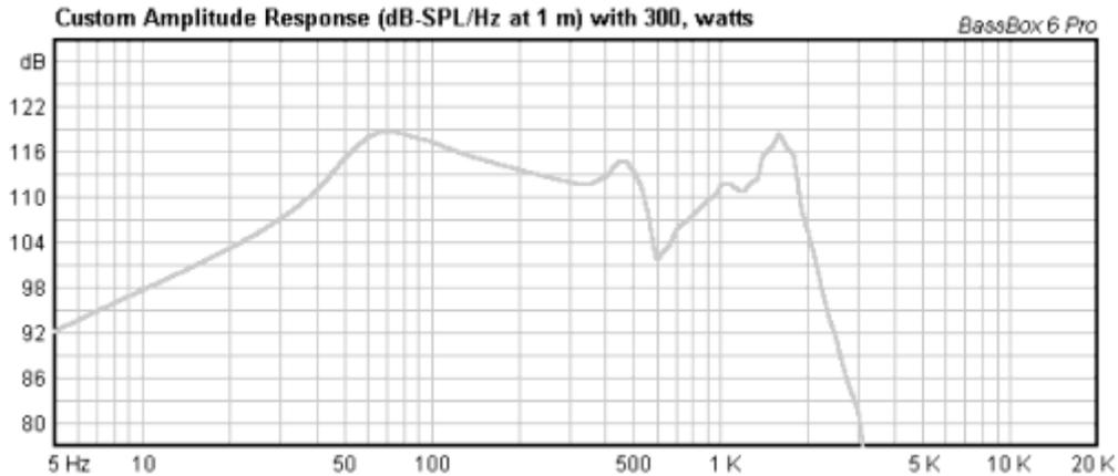
From the simulation can be seen that very high SPL close to 119 dB is possible from 60 to 100 Hz.
