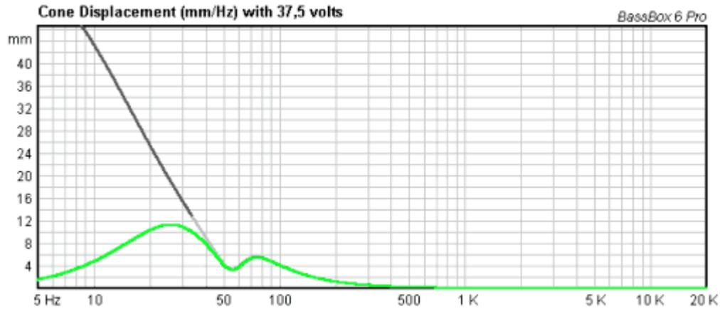
As seen above the high pass filter greatly reduces cone displacement below tuning. Further bass extension (red curve) can be obtained in a 35 litre box using the same port dimensions as for the 28 litre box above.
