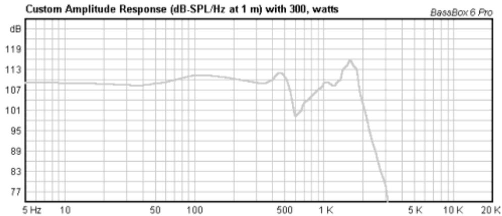
This simulation says that around 60 Hz the sound pressure in 1 meter distance is approximately 110 dB from a 14 liter box.
