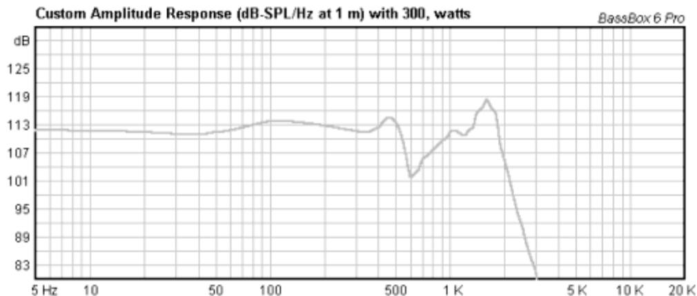
It can be seen that low bass extension is possible in a small sealed box.
